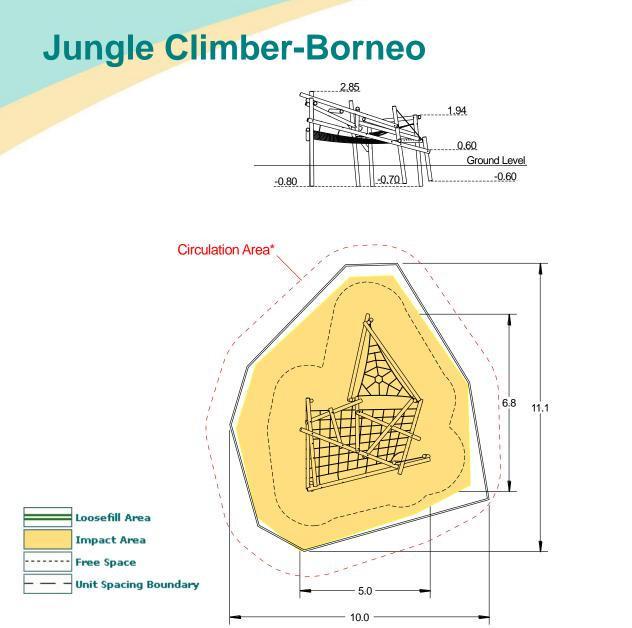
\* Recommended Circulation Area (1.2m outside impact area) – this area should be clear of solid raised objects (ie.fences, walls, trees and other items of equipment). Loose fill retaining edgings are acceptable in this area.
